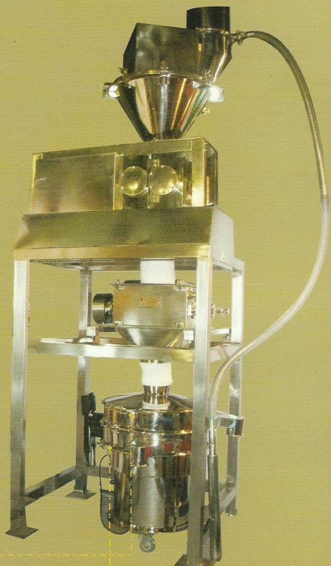
Producing granules of higher Bulk Density & better flow ability
